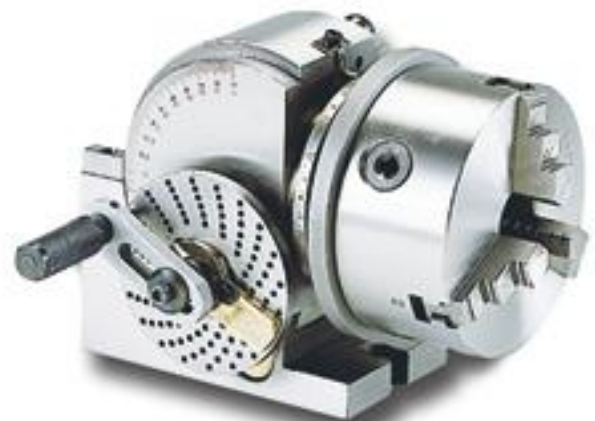
The state of BS-0 fitted with 5" 3-Jaw Chuck
